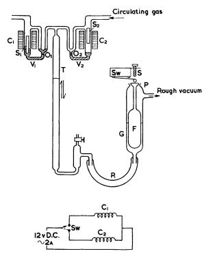
robust and reliable in operation, and gives positive and measurable rates of gas circulation, from pressures of at least 76 cm. to well below 0.1 mm. (*i.e.*, down to pressures at which diffusion becomes important) without any alteration or adjustment except of the level of the reservoir G.
